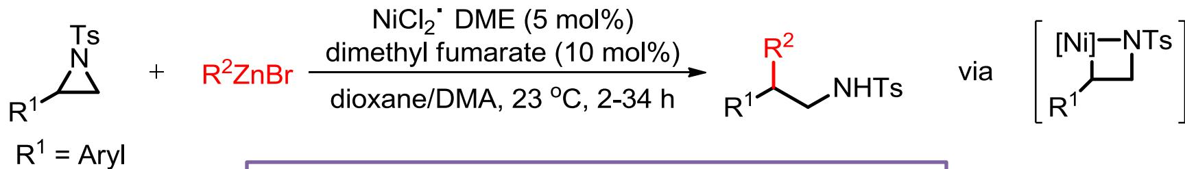
Dimethyl fumarate: accelerate reductive elimination through  $\pi$ -coordination to nickel
